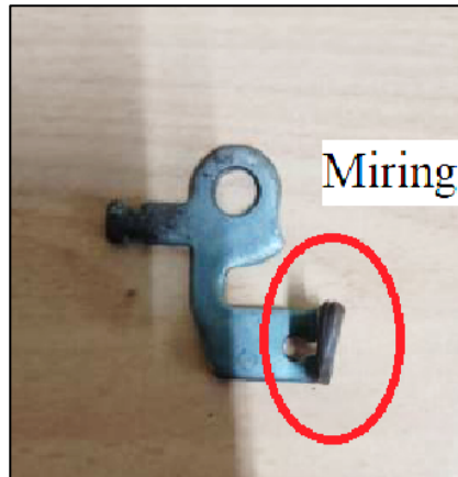
Gambar 4.15 Cacat Tilt (Miring)
