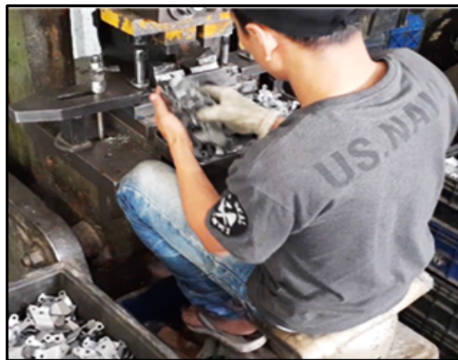
Gambar 4.5 Proses Setup material sebelum proses Shearing
