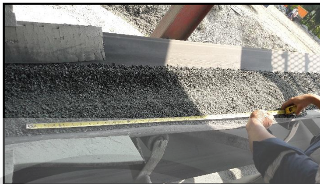
Gambar 4.6 Foto Pengambilan Material Belt Cut
