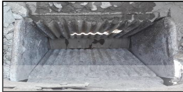
Gambar 4.9 Foto Feed Opening dan CSS Primary Jaw Crusher
